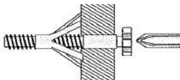
For use with plaster board partitions or hollow wooden doors.
